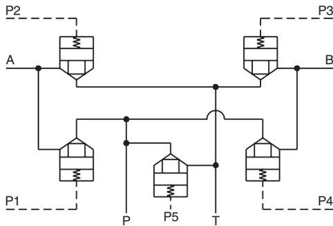
*Circuit 2, with \*\*SLC2A/R0\*E3 spool logic elements.*
