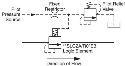
**Pressure relief or sequence example with internal pilot supply and pilot relief.**
