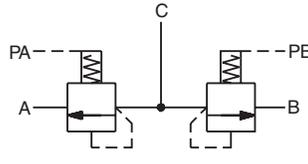
*Circuit 3, with \*\*SLC2A/R0\*E3 spool logic element.*
