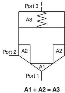
Poppet type logic valves are 3 ported, 2-way on/off valves that switch flow between port 1 and port 2. The poppet's on/off action is operated by controlling pilot oil at port 3 of the valve. A small low flow solenoid or pilot valve is an ideal control for this purpose. Parker offers vent-to-open and pilot-to-close style poppet logic valves.
