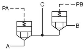
*Circuit 2, with \*\*SLC2A/R0\*E3 spool logic element.*
