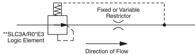
**Load sensing priority flow control example with pressure limiting and unloading.**
