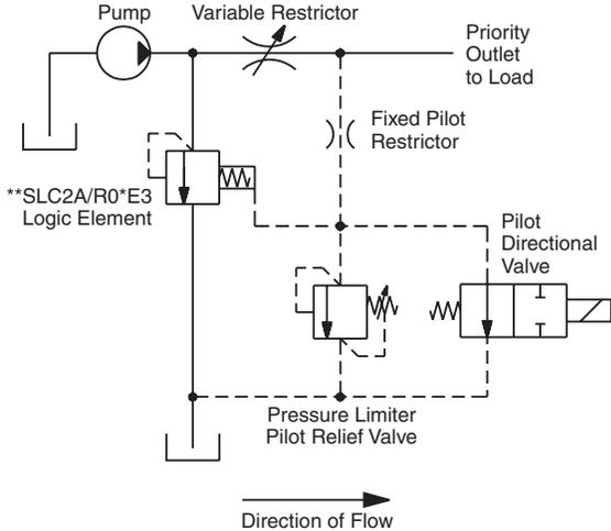
**Load sensing priority flow control example with pressure limiter.**
