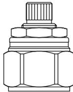
**Knob Adjustment** - An aluminum knob is added to the standard screw adjustment. A lock knob is provided to help maintain the desired setting after adjustment. Parker offers knob conversion kits for most pressure control valves. For kit numbers consult individual valve pages.
