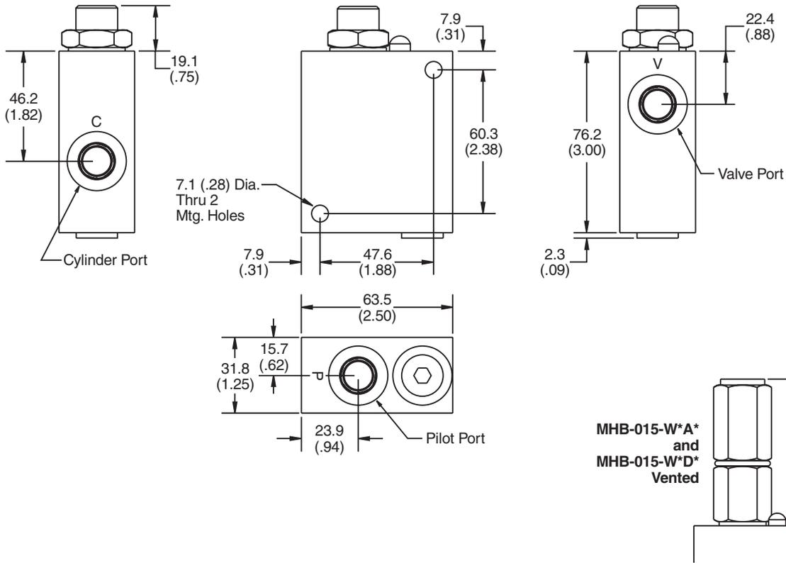
**Series MHB-015-L\*D\*** Dual Counterbalance, Non-Vented, In-line Mount
